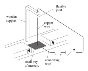
The teacher sets up the apparatus in a fume cupboard because mercury vapour is poisonous. Draw arrows on the diagram to show the direction of
